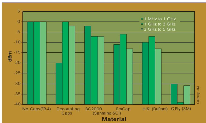
Figure 3 – A comparison of powerbus noise for a test circuit with no caps, discrete decoupling caps and several different distributed capacitance materials
