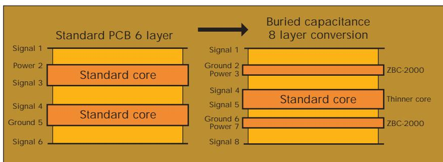
**Figure 1** – Adding capacitance with thin dielectric power/ground planes
