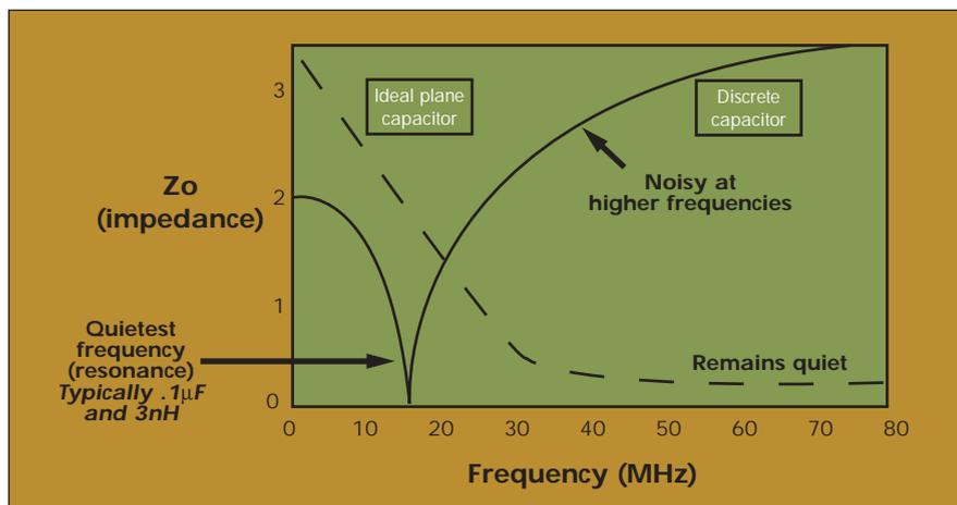
Figure 2 – Resonant discrettes vs. nonresonant plane bypass capacitor impedance
