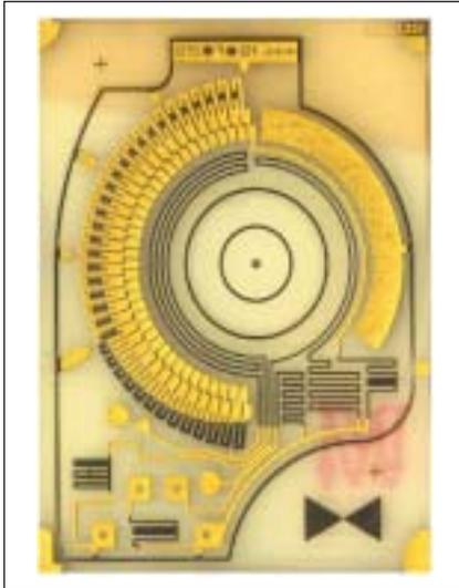
**Figure 5** – Circuit for a camera, with resistors forming a rheostat type of pattern
