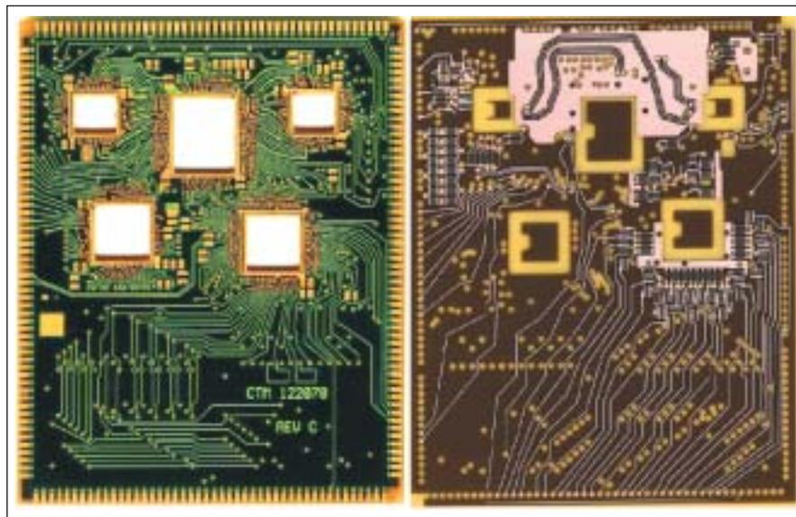
**Figure 4** – Outer- (left) and innerlayer (right) of a probe card with buried passives. To reduce signal path, resistors are placed directly under component leads
